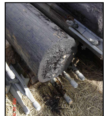
Typical wood pole leaching dangerous chemicals
